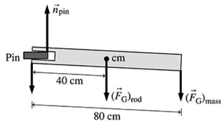
As the gravitational force on the rod and the hanging mass pull down (the rotation of the rod is exaggerated in the figure), the rod touches the pin at two points. The piece of the pin at the very end pushes down on the rod; the right end of the pin pushes up on the rod. To understand this, hold a pen or pencil between your thumb and forefinger, with your thumb on top (pushing down) and your forefinger underneath (pushing up).
